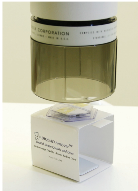
Figure 1. An Analyzer for evaluating intraoral image quality and patient dose. It consists of a cube (approximately 2"), a radiation dosimeter and test patterns (on top), and a dental film packet containing D- and F-speed films. For digital systems the sensor is placed on top of the film packet.
