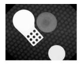
The structured noise (dotted or honey comb pattern in the darker areas of the image) is due to replacing a sensor without recalibrating the imaging system.
