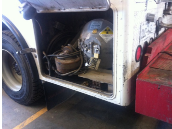
Figure G-3 Storage compartment with a permanently mounted transport shield
